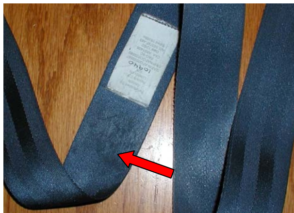
Figure 13: “Scratched” – minor surface scratches and scuffs on webbing exterior
