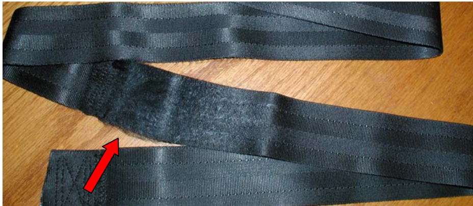
Figure 4: “Very Frayed” – exterior of webbing is substantially worn and damaged
