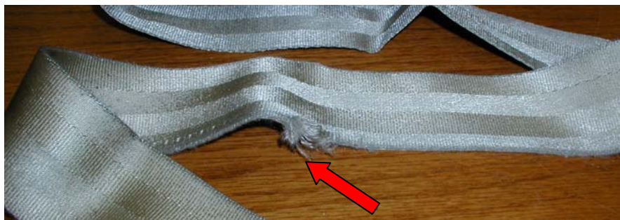
Figure 5: “Small Rip” – torn less than 0.5 inches on edge of webbing
