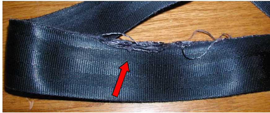
Figure 6: “Ripped” – torn between 0.5 and 3 inches on edge of webbing
