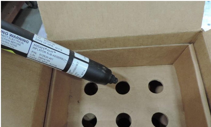
EXAMPLE – INSERT INFLATOR DIFFUSER-END DOWN (POLY BAGS REMOVED FOR CLARITY)
