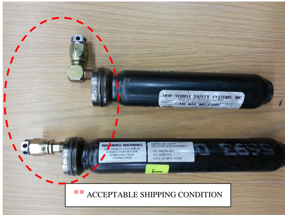
STAGED SHIPPING CAP INSTALLATION - BOTTOM, FINGER-TIGHT IS ADEQUATE -
