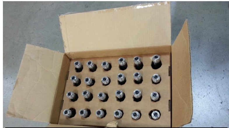
EXAMPLE 24-CELL – TOP VIEW – IGNITER-END UP (FOAM PAD AND POLY BAGS REMOVED FOR CLARITY)
