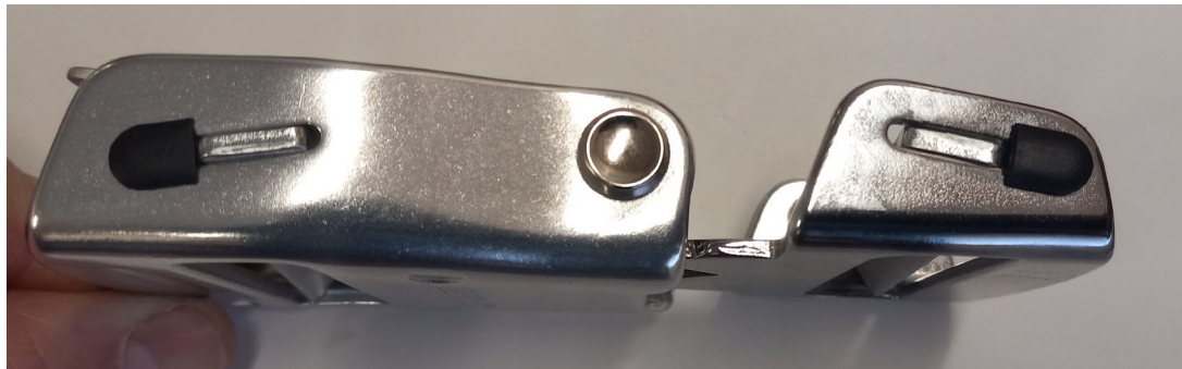
Figure 2. Buckle/Connector with Incorrect Plug Installation
