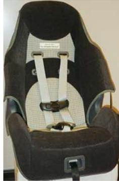
**c. Non-Approved “Booster Seat.”** The CRS in the following image (CRS without Internal Restraint Marketed as a Booster Seat) would not be approved for use during all phases of flight.
