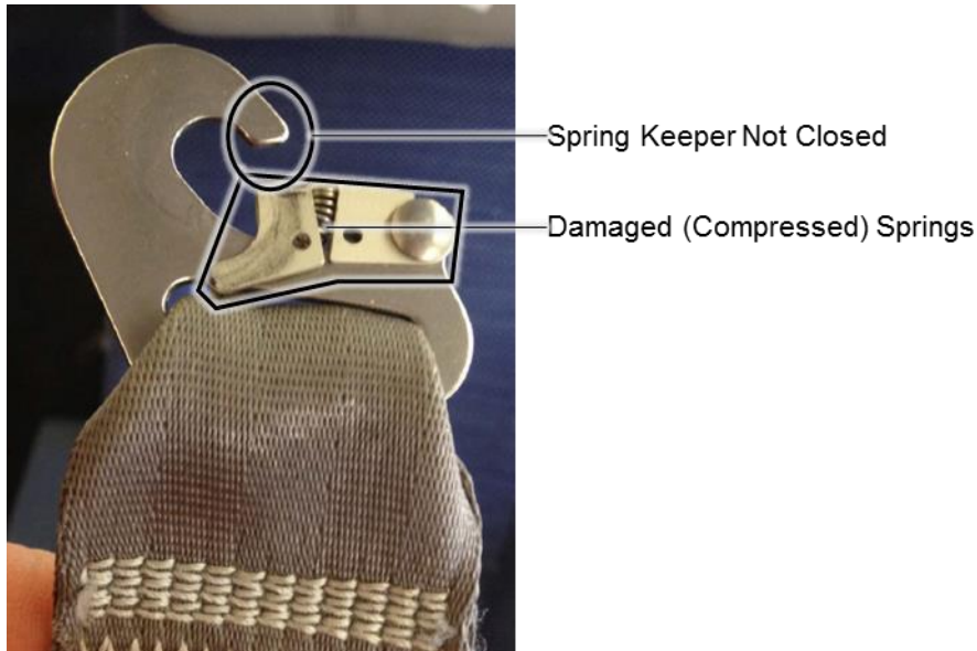
Figure 4 – Damaged Hook Assembly
