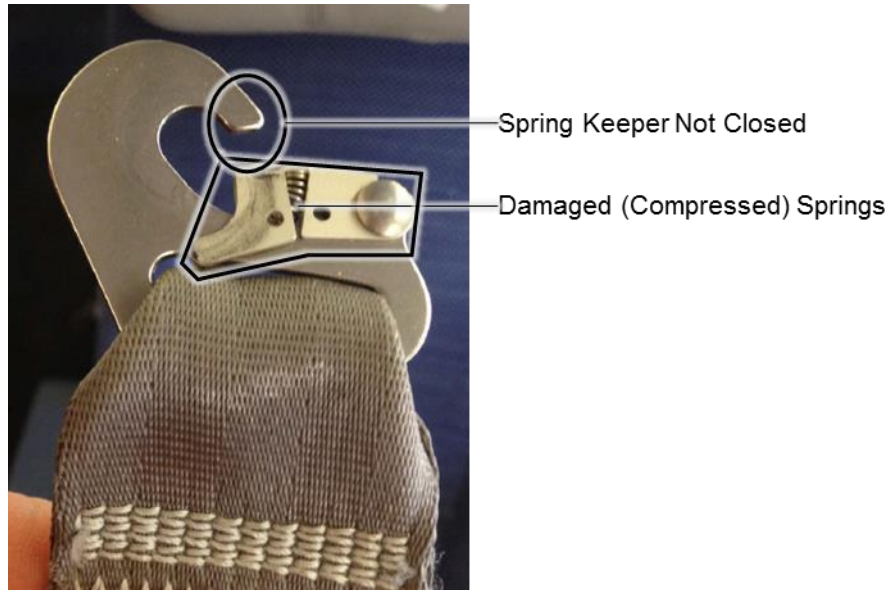
Figure 4 – Damaged Hook Assembly
