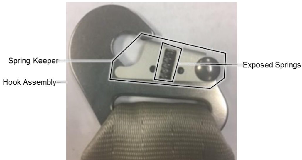
Figure 2 – Hook Assembly With Exposed Springs
