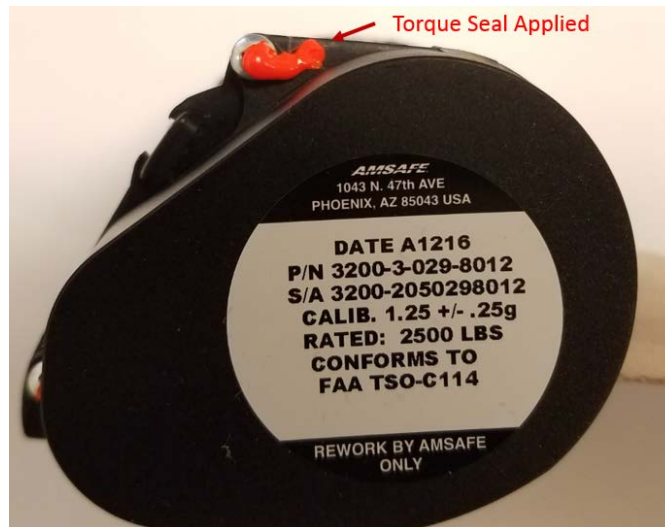
Figure 4: Torque Seal Applied to Upper Fastener (Dust Cover Shown)
