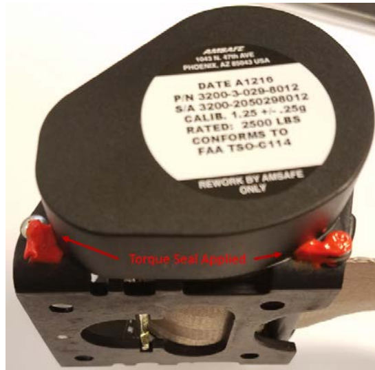
Figure 3: Torque Seal Applied to Lower Fasteners (Dust Cover Shown)
