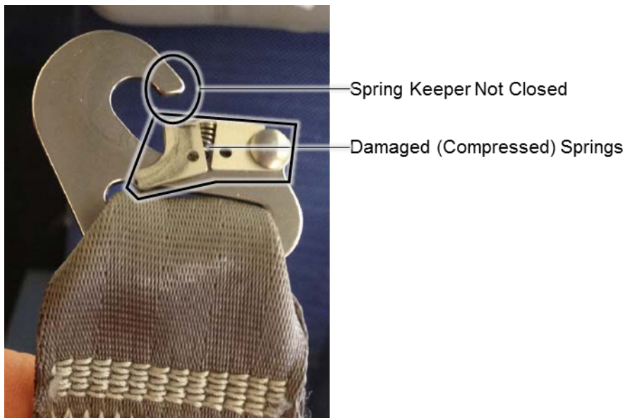
Figure 4 – Damaged Hook Assembly
