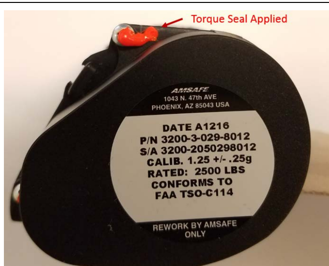
Figure 3 – Torque Seal Applied to Fastener C
