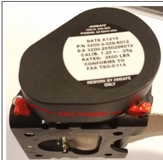
Figure 2 – Torque Seal Applied to Fasteners A and B
