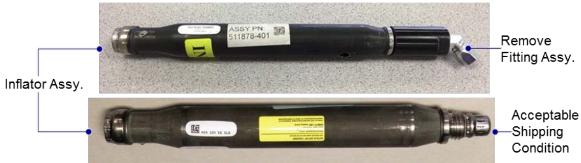
Figure 12 – Example Fitting Assemblies and Inflator Assemblies
