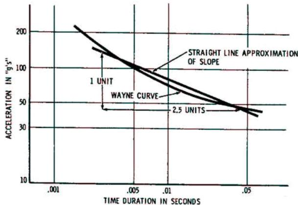
Figure 1: HIC Based on Injury Tolerance Curve
