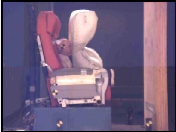
Figure 5: Static Deployment with Three Year Old ATD
