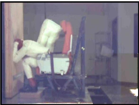
Figure 6: Static Deployment with 50% ATD In Brace Position
