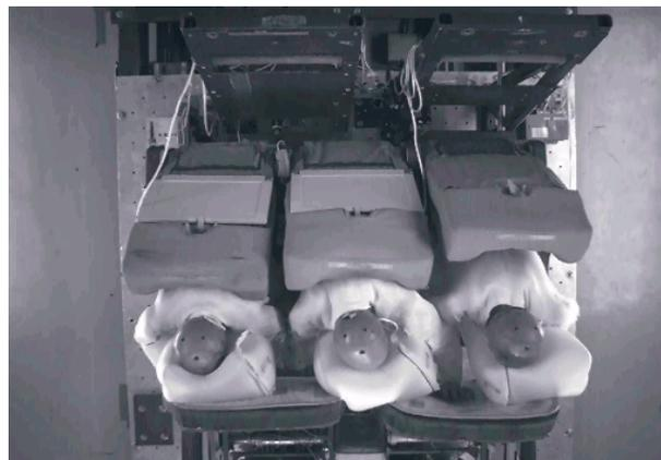
Figure 3: Row to Row 16G Test with AAIR
