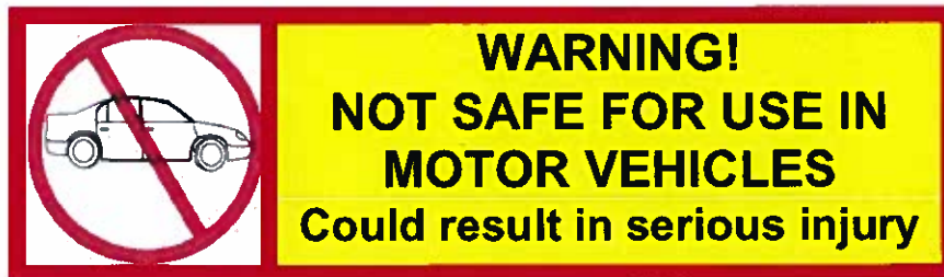
FIGURE 1. REQUIRED WARNING LABEL FOR AVIATION CHILD SAFETY DEVICES WITHOUT FMVSS NO. 213 APPROVAL
