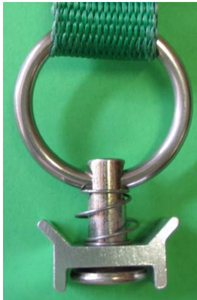
Single Stud Fitting No Damage to Spring
