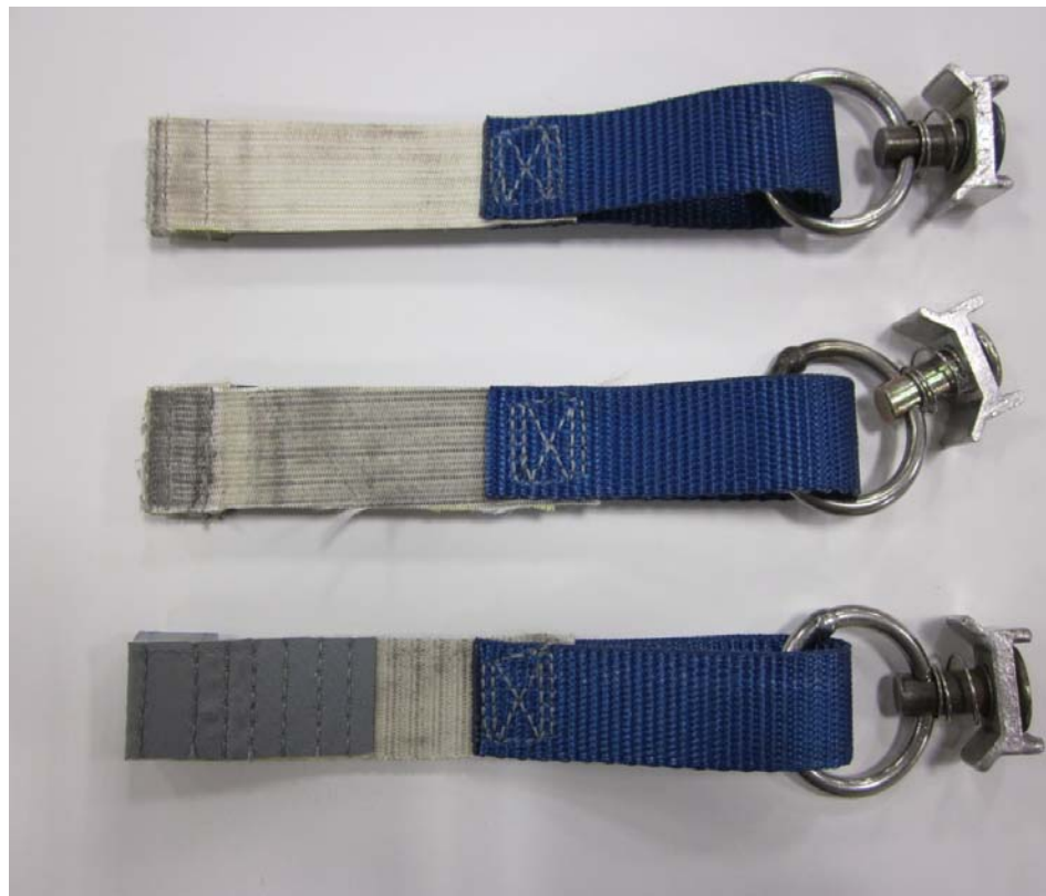
Test samples before pull testing. (Top to bottom – New, Used, and Repaired)
