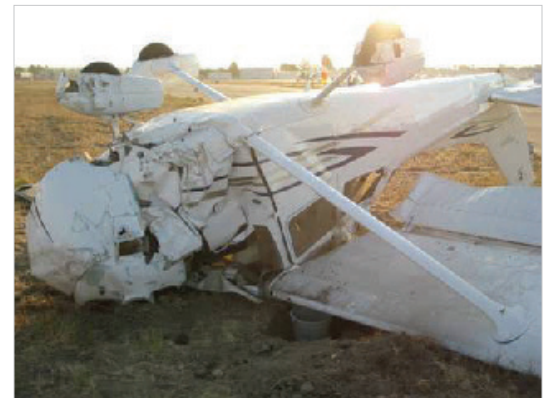
Aircraft sustained typically non-survivable impact. Airbag deployed and although the pilot sustained severe injury, he survived. Photo courtesy of AmSafe.
