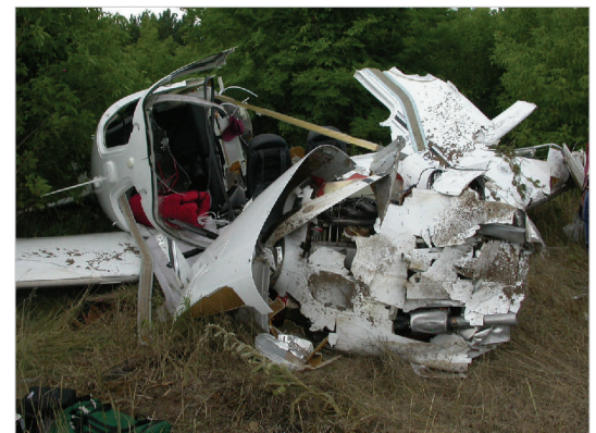
Aircraft stalled and cartwheeled. The aircraft was destroyed, but the airbags deployed and the occupants evacuated without life-threatening injuries. Photo courtesy of AmSafe.
